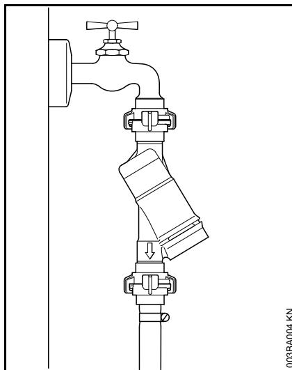
When hooking up to the drinking water main, a backflow preventer must be installed between the water tap and the hose. The design of the backflow preventer must comply with the applicable country-specific regulations.
