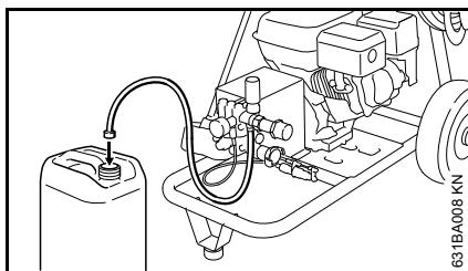
With the intake hose, detergent can be drawn in and added from a separate container.
